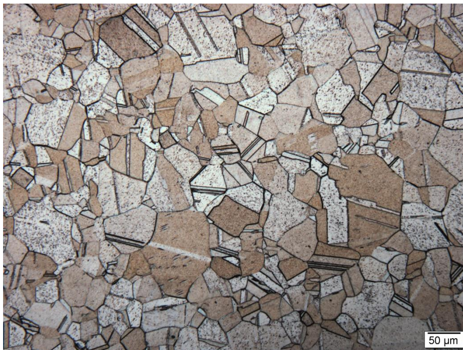
Figure 26 - AISI 304 steel micrograph, after recrystallization. Electrolytic Etching with \text{HNO}_3 , followed by etching using modified Beraha II. Parameters: 15 s and 1.1 A. Using Nomarski filter.
