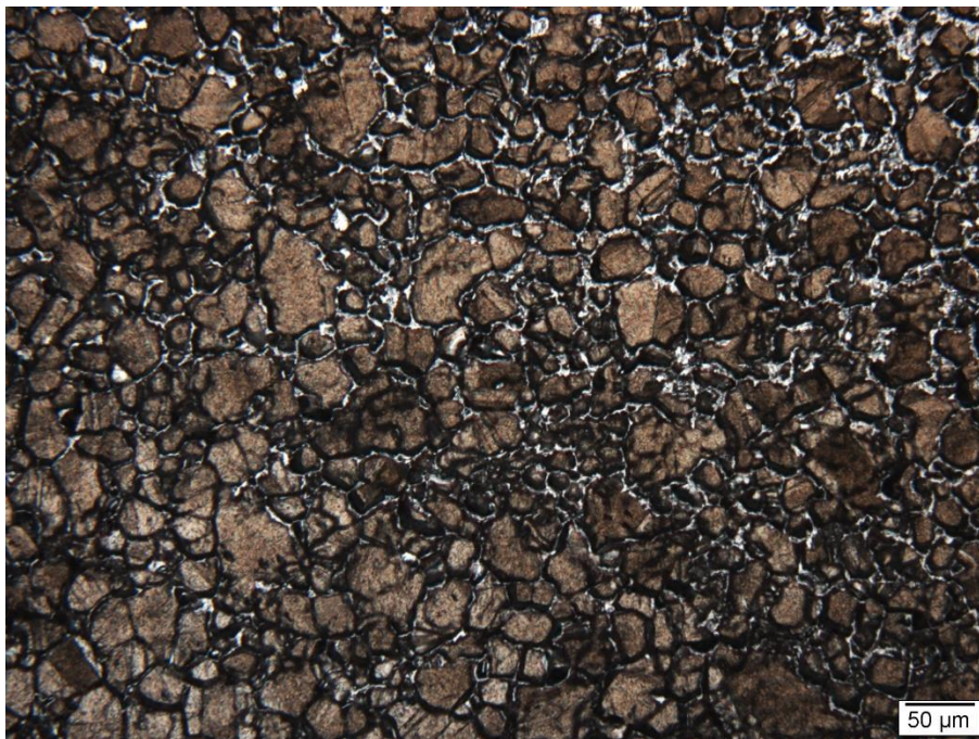
Figure 25 - AISI 304 steel micrograph in regions with strong corrosion effect. Electrolytic Etching with \text{HNO}_3 . Parameters: 25 s and 1.1 A. Using Nomarski filter.
