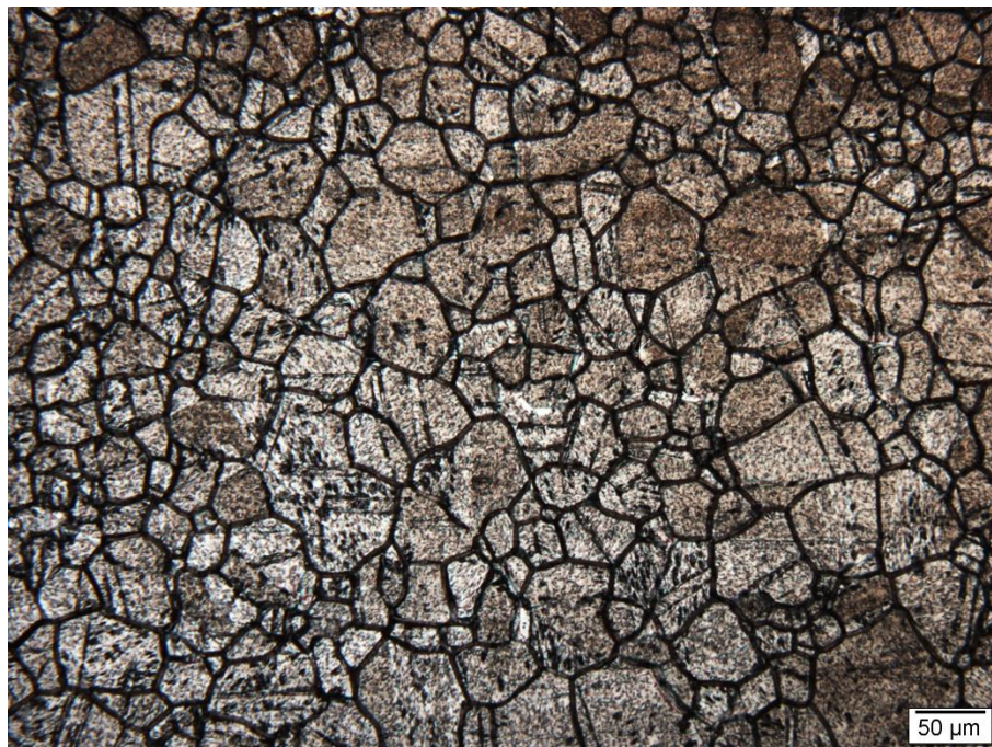
Figure 24 - AISI 304 steel micrograph, after recrystallization. Electrolytic Etching with \text{HNO}_3 . Parameters: 25 s and 1.1 A
