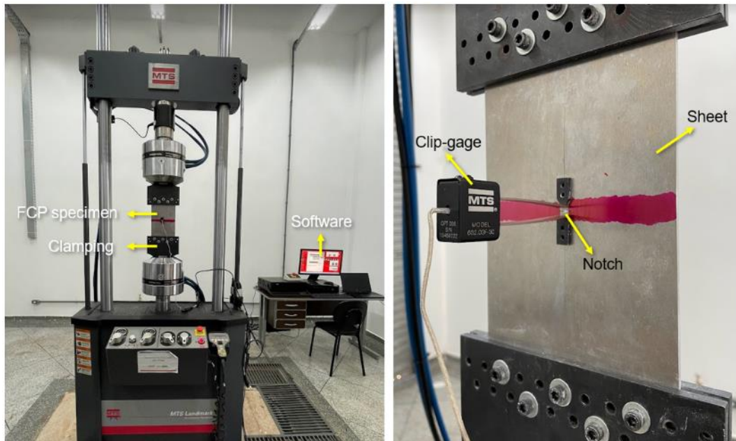
Figure 38 – Servo hydraulic machine MTS by Landmark, specimen, clamping and clip-gage system.
