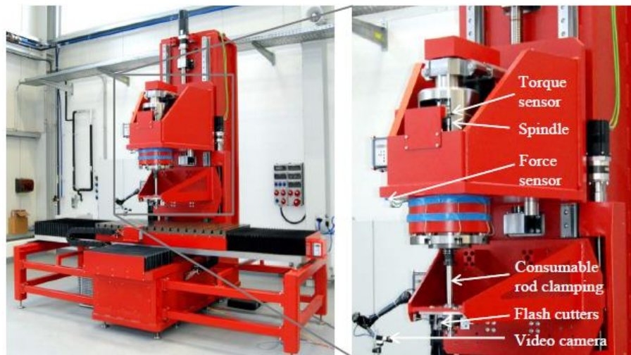
Figure 29 – Illustration of HLR RAS 1 machine used to produce layer FS deposition process at Hereon (Germany).
