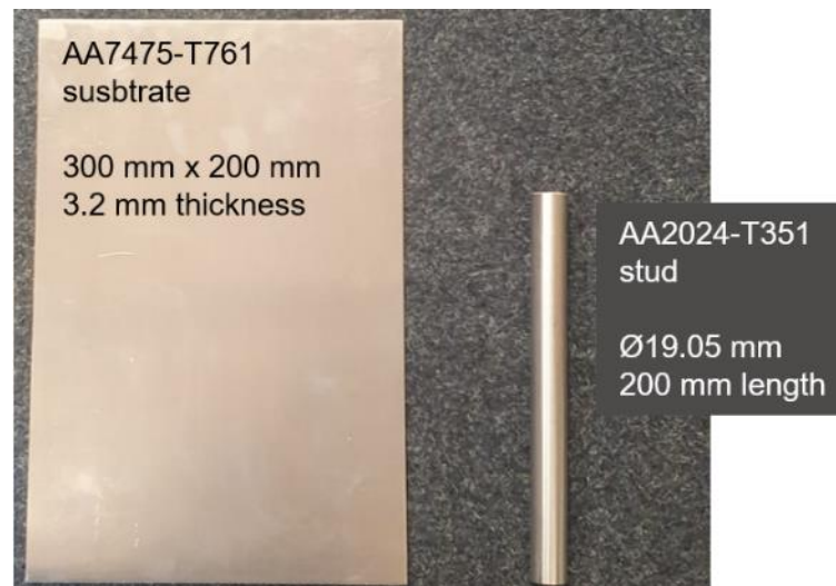
Figure 28 – AA7475-T761 substrate and AA2024-T351 stud material provided by EMBRAER SA.
