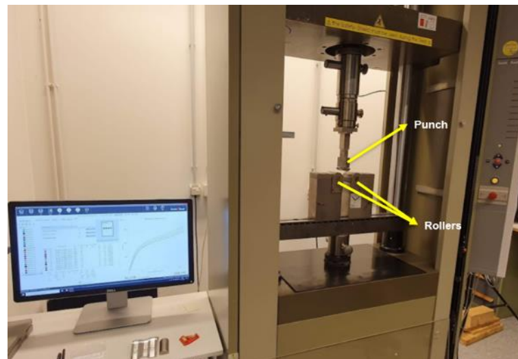
Figure 33 – Universal testing machine used for three-point bending test at Hereon (Germany).
